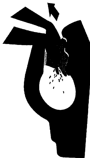
Figure 1 Simplified view of moisture being 'stripped' from the hands by the air knives of the Dyson Airblade™ hand dryer.
