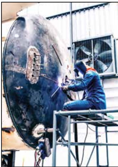
This employee must wear protective clothing while working with welding* equipment*. Bigstockphoto.com
