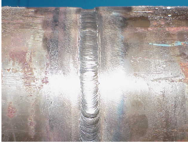
5G Position Pipe axis is parallel to the horizontal plane and the pipe is not rotated
