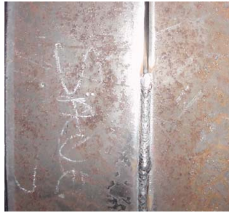
An example of a high quality root pass.
