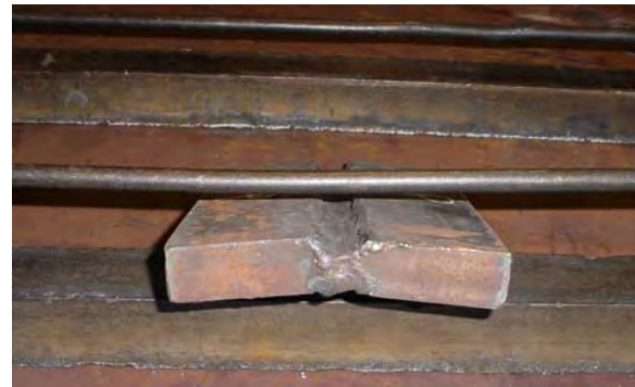
U-Shaped groove by carbon arcing
