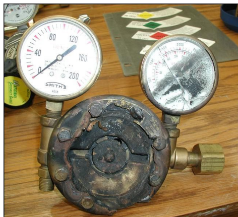
Regulator Blow Out (also known as a Valve Seat Fire)
