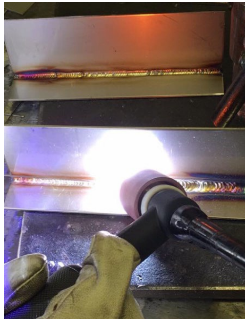
Example of a High-Quality Welds Weld Quality per Industry Standards
