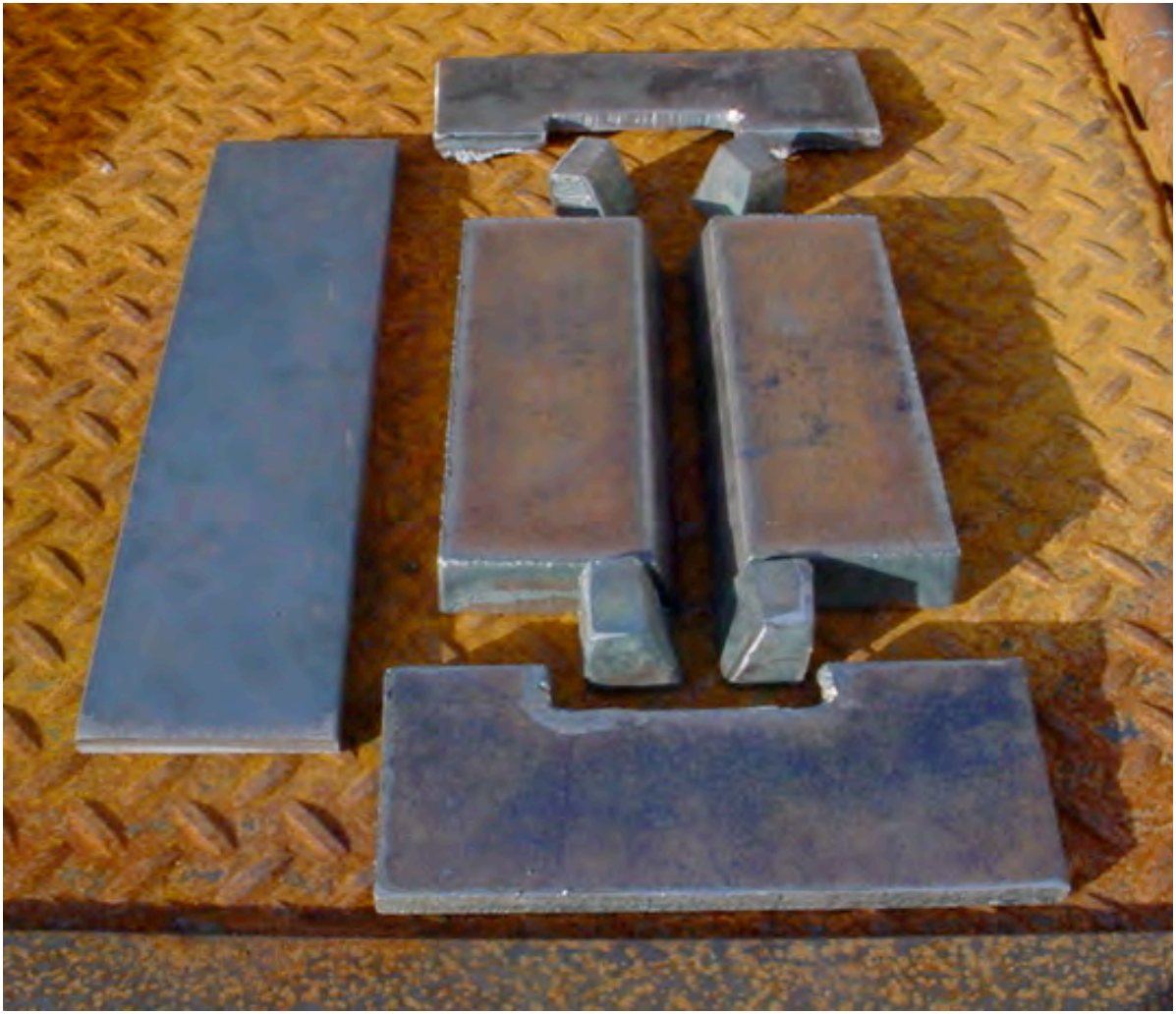
All the pieces needed to assemble a Single V Groove Weld with Strong Backs.
