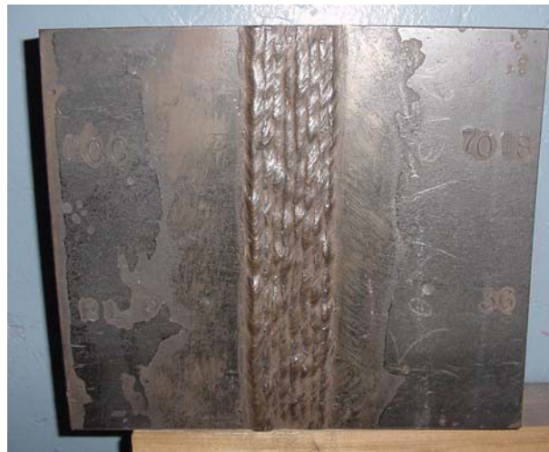
Example of a High Quality Weld
