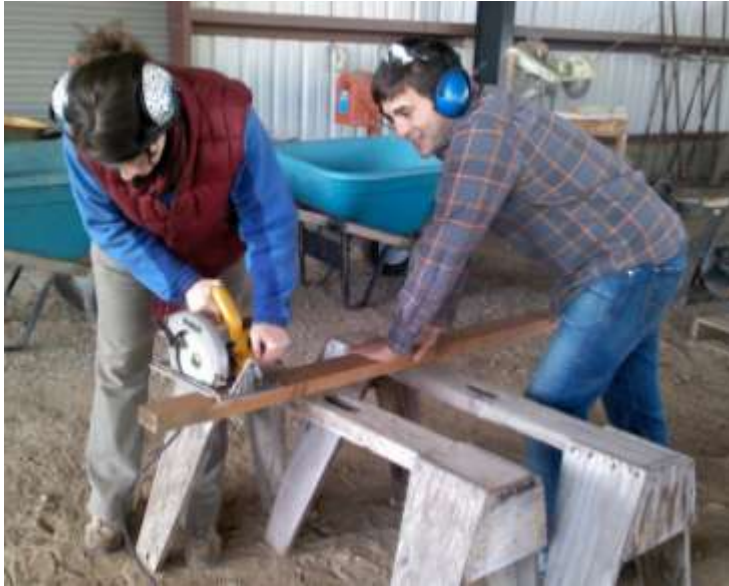
Figure 1. Making a crosscut with a circular saw.
