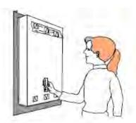
12. Once every hour for a few hours on a cloudy day, and for a few hours on a sunny day, hold the thermometer under the plastic flaps covering the vent holes for 2 minutes to measure the collector's air intake (bottom) and output (top) temperatures. Mark your temperature readings on the graph paper.
